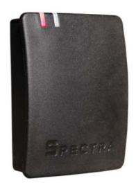
P20 Proximity reader is indigenously developed high performance reader to read EM RFID read only card. It provides a consistent read range of 8~10 cm in most of the conditions. The reader is particularly suited to access control applications. The same basic unit can be configured to most common output interface formats, including Wiegand, Magstripe and RS-232 serial ASCII.
